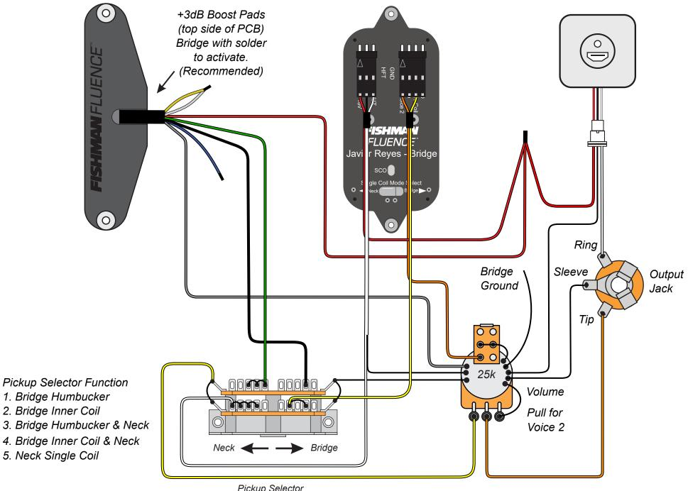
Pickup Selector 4-Pole 5-Position Switch
