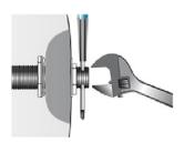
Thread and gently tighten the strap button using rubber tipped pliers
