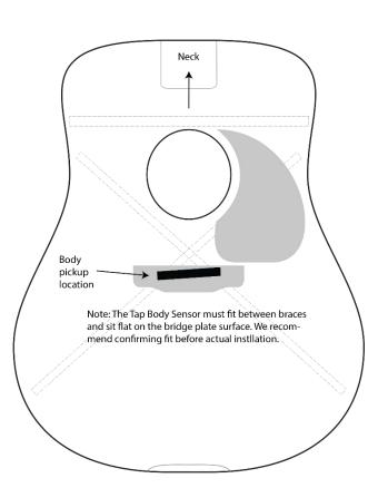
Use the included mounting tool and two golf tee locaters to ensure proper placement of the Tap Body Sensor.
