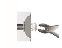
Note: With the strap button in place, the end of the jack should protrude slightly, so that when a plug is inserted, it will snap securely in place.
