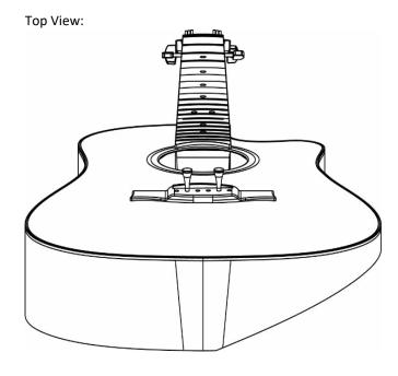
2. Using one of the golf tee locator pins, insert it through the "A" string bridge pin hole and into the round hole in the corner of the mounting tool. Using the second golf tee, insert it through the "B" string bridge pin hole and into the slotted hole in the opposite corner of the mounting tool.
