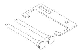
To properly mount the Tap Body Sensor, insert it as shown into the mounting tool.
