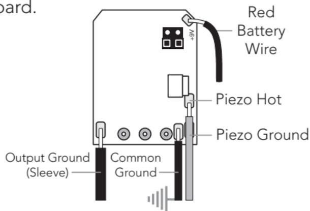
3. Solder the magnetic pickup hot wire to the circuit board.
