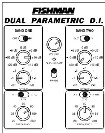
If you want to boost the low-end response for a bass drum while de-emphasizing any ringing, you can separately boost and cut using Band One and Band Two as follows (the frequencies are merely examples-experiment with your own combinations):
